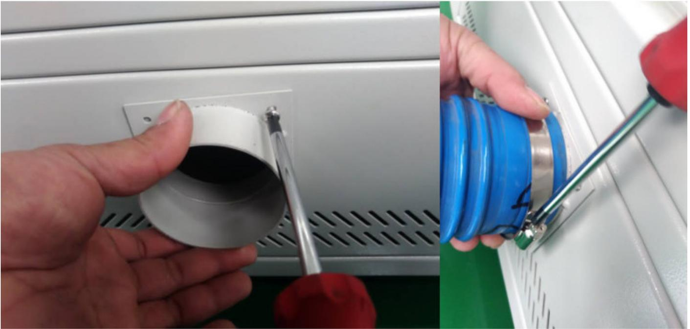
Screw in the exhaust pipe fixture, fasten the rings after you put on the pipe on the fixture. Lead the other end of the pipe outside your windows or house ventilation
