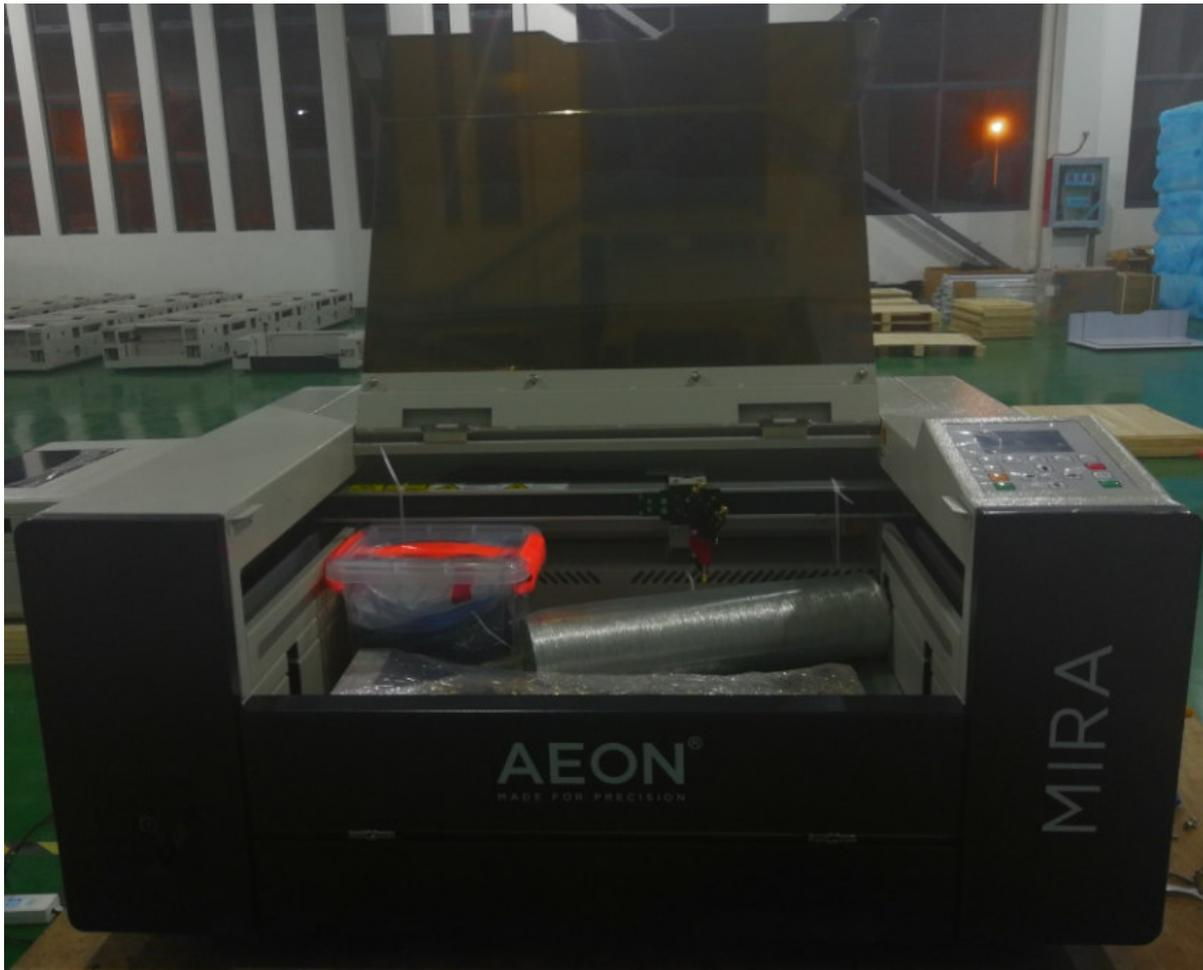
The gantry of the machines are tied by the binder. You have to cut it before running the machine!
