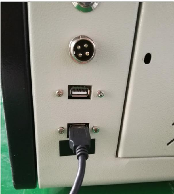
The USB interface is used to connect data cable, which you could connect the data cable to computer. Or you could connect WIFI if your machine got WIFI. There are WIFI setting instruction in the following Chapter
