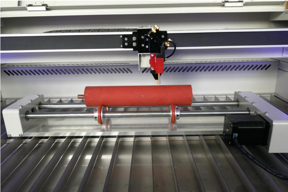
Plug the rotary device into the rotary port we left on the right of the machine:
