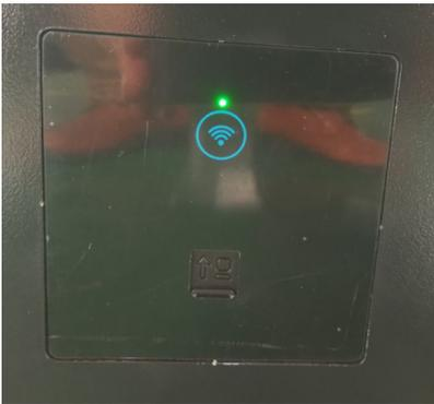
Built in WIFI is installed on the down left corner of the machine. When the green light is blinking, the WIFI is available. You can go to computer to check and connect the WIFI.
