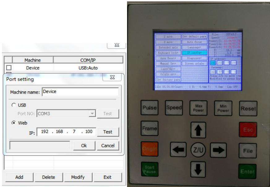
Lastly, click the 'Test' to test the connection, it shows port test successful, then you can click “确定” to quit and then WIFI setting is ready.
